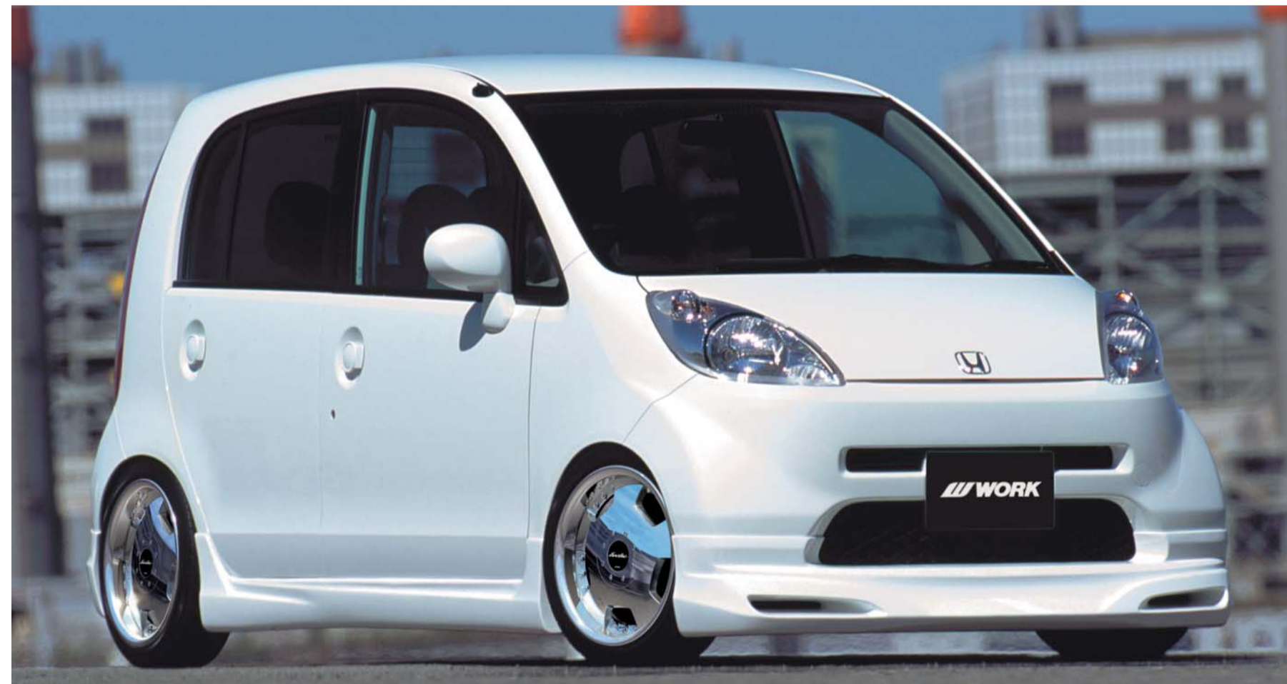
[SIZE] FRONT:15inchX5.5JJ OFFSET +35mm(O) TIRE:165/45-15 REAR:15inchX5.5JJ OFFSET +35mm(O) TIRE:165/45-15 COLOR:クロームメッキ (M) ※フエンダー加工
