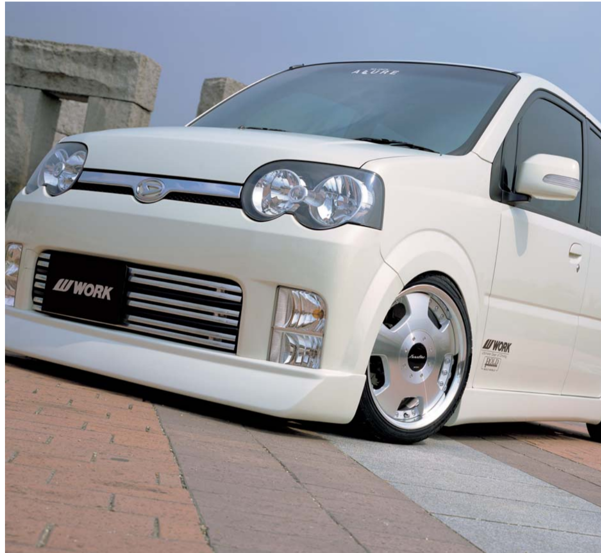
[SIZE] FRONT:16inchX6.0JJ OFFSET +38mm(O) TIRE:165/45-16 REAR:16inchX6.0JJ OFFSET +25mm(A) TIRE:165/45-16 COLOR:カットクリア (SP) ※フエンダー加工
