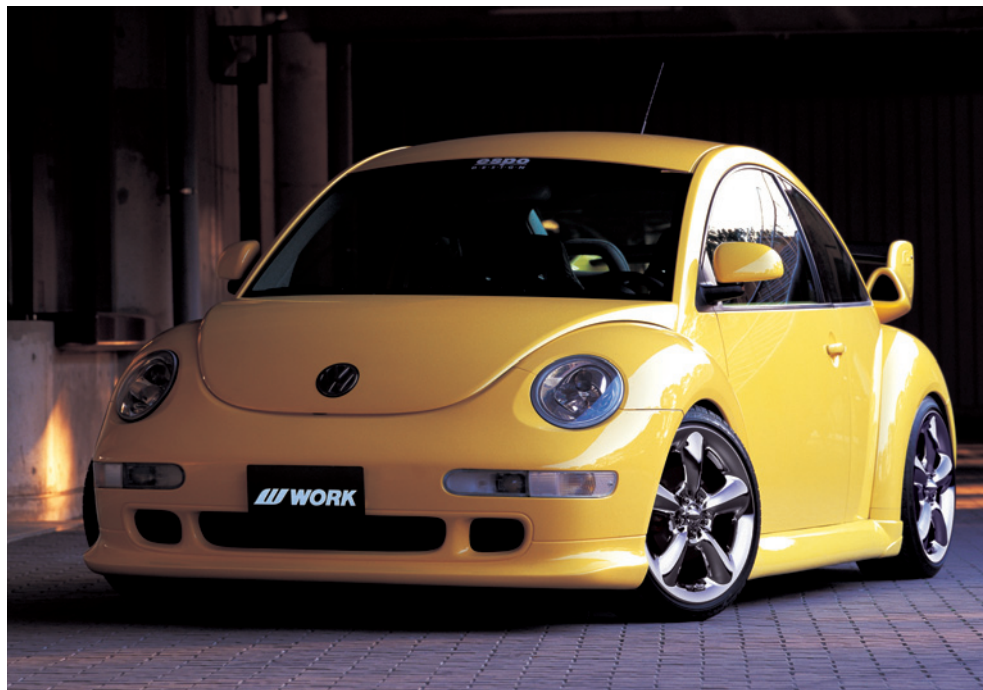
[SIZE] FRONT:18inch×8.0JJ INSET38mm TIRE:215/40-18 REAR:18inch×8.0JJ INSET38mm TIRE:215/40-18 COLOR:クロームメッキ (M) ※フェンダー加工
