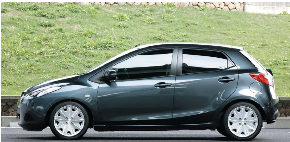
[SIZE] FRONT:16inchX6.5J OFFSET +38mm TIRE:195/45-16 REAR:16inchX6.5J OFFSET +38mm TIRE:195/45-16 COLOR:カッタクリア (MSP) ※フェンダー加工
